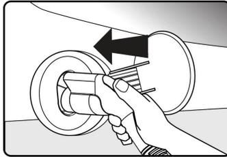
5. **Automatic charge begins.** Power will be delivered in accordance with vehicle demand. If the vehicle is charging, the **BLUE STATUS Indicator** will blink on and off approximately every two seconds. Always verify that the vehicle charging status indicator agrees.
